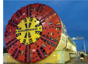
- Diameter: 15,200 mm - Cutter head Power: 12 MW
