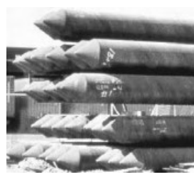
(g) Timber pile toe
