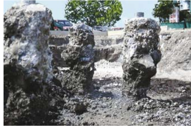
Test site: grouted driven piles after removal of soil nail around them
