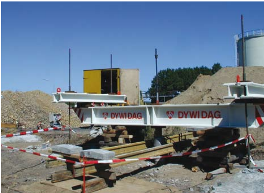
Static pile test
