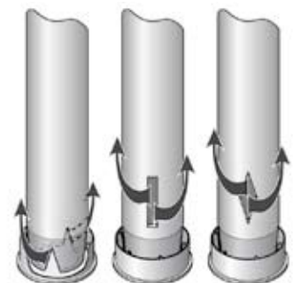
Cutaway above grout shoe for grouted piles
