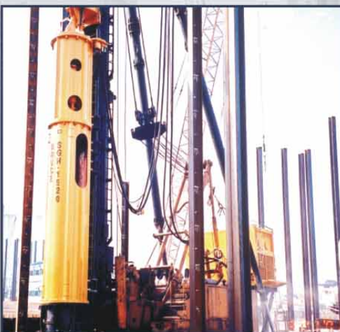
SGH-2015 20ton RAM WEIGHT with 1.5m STROKE
