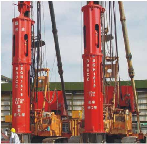
SGH-1619 HIGHEST RAM STROKE with 1.9m STROKE
