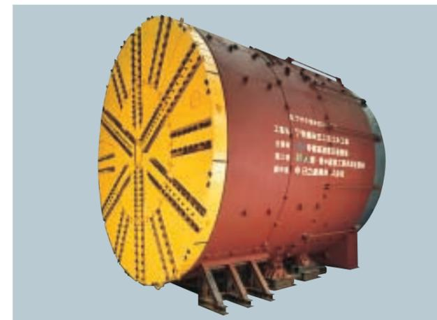
9.7 m dia. slurry shield (for subway)
