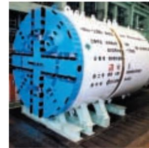
4.5 m dia. receiving slurry shield
