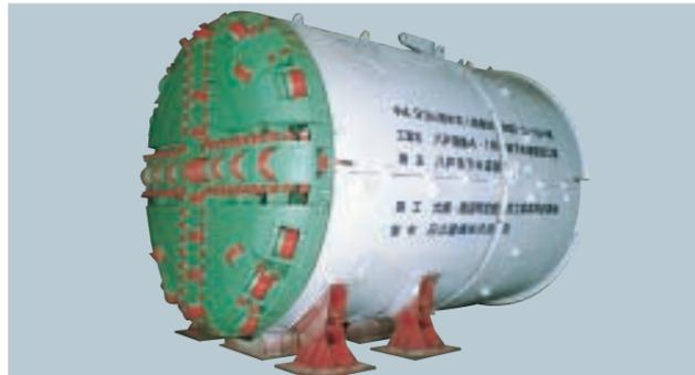
**4.93 m dia. earth pressure balanced shield**
