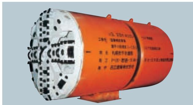
**3.28 m dia. earth pressure balanced shield**
