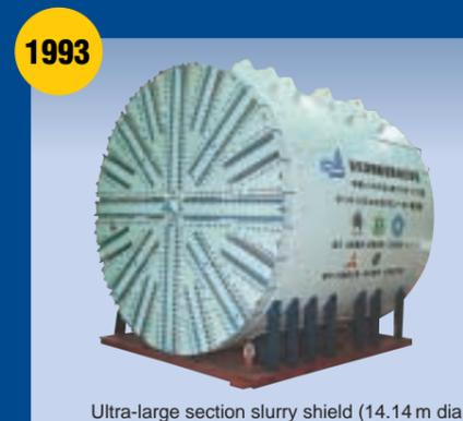
Ultra-large section slurry shield (14.14 m dia.)
