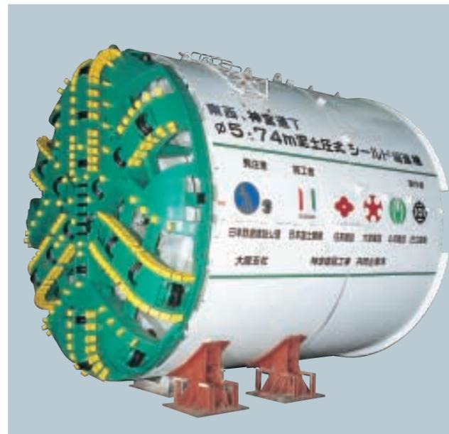
**5.74 m dia. earth pressure balanced shield**
